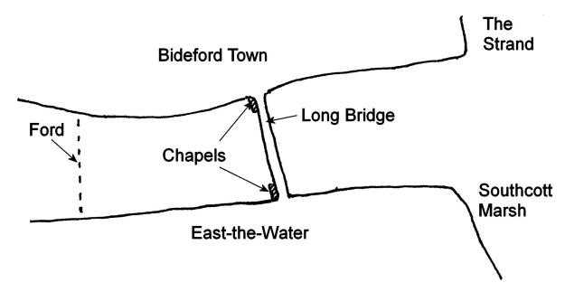
Ascott notes that the bridge was originally slightly convex down the river to resist the force of the incoming tide<sup>128</sup>.
